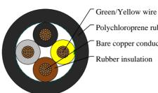
Polychloroprene rubber outer jacket Bare copper conductor
